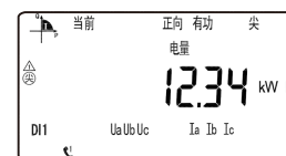
Current forward active energy 12.34kWh
